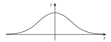
The graph is formed from two convex sections, where the gradient is increasing, and one concave section, where the gradient is decreasing.
